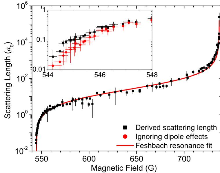
Fig. 6. Scattering length  $a$  vs.  $B$ . The inset shows the zero-crossing in detail. The squares are the extracted values of  $a$  when the magnetic dipole interaction is accounted for, while the circles correspond to its neglect.
