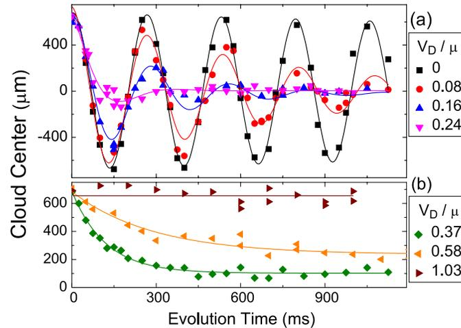
Fig. 4. Damping of dipole oscillations for various  $V_d$ . Reprinted from Ref. 12.
