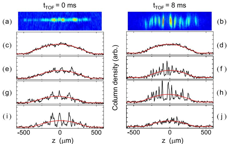
Fig. 5. *In situ* (left) and TOF images (right) for various  $V_d$ . (c, d)  $V_d = 0$ ; (e, f)  $V_d \approx 0.3\mu$ ; (a, b, g, h)  $V_d \approx 0.5\mu$ ; (i, j)  $V_d \approx 1.0\mu$ . Reprinted from Ref. 12.
